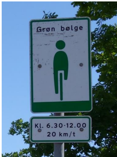
Figure 5. "Green wave" for cyclists, with traffic lights synchronised for 20 km/h in the direction of the city centre in the morning. Copenhagen, Denmark.
