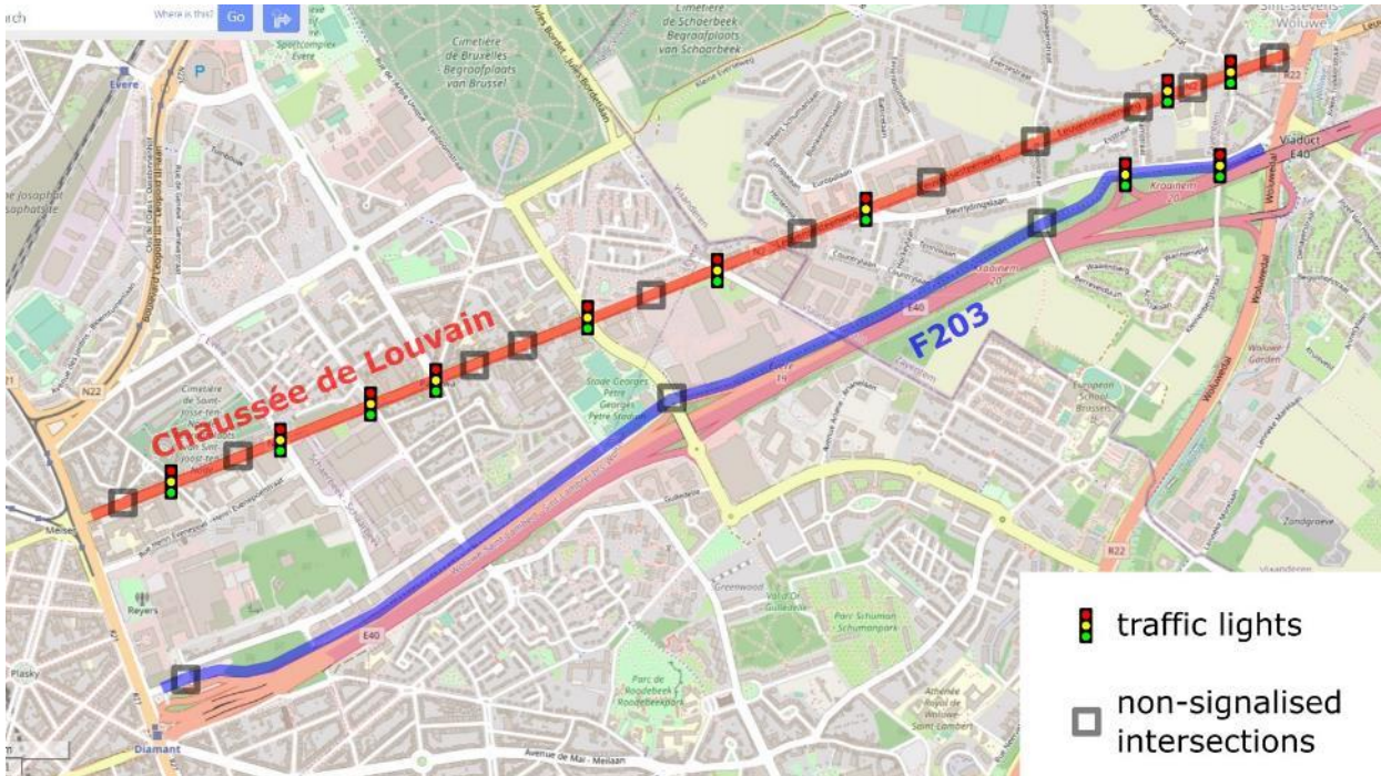
Figure 3. Signalised and non-signalised intersections in two parallel corridors in Brussels: Chaussée de Louvain (distributor road) and F203 cycle highway. Background credit: OpenStreetMap.
