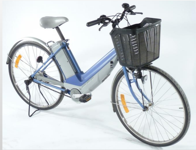
1993 Yamaha PAS Electric bicycle with pedal sensor controlled power assist system
