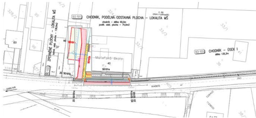
Figure 14 - Official project map (doc3) showcasing "Grass-grid concrete paving (parking area)" (yellow); "Concrete paving thickness 8cm (driveway)" (red) and "Concrete paving thickness 8cm (parking area)" (gray). [(1_3)doc3]
