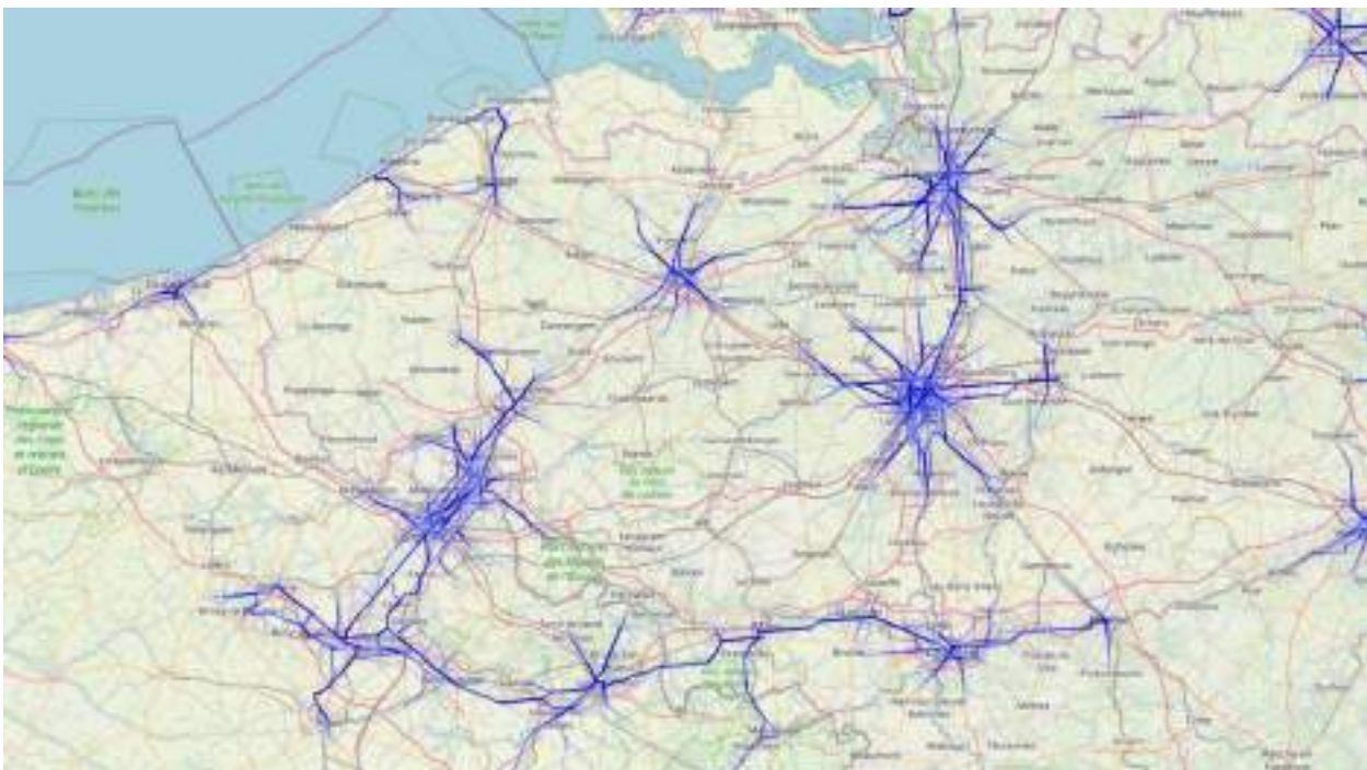
Figure 50. Cycle Highway Potential Map, developed in the frame of the CHIPS project, is a simple EU-level model evaluating the potential for medium-range cycle trips on the basis of the Eurostat demographic data.
