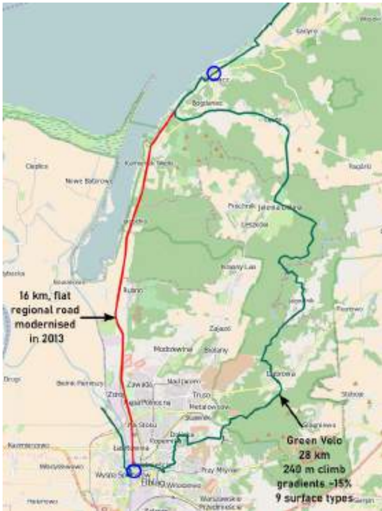
Figure 30. The Green Velo route leaving Elbląg follows a complicated route through the hills, resulting in detour factor close to 2, gradients up to 15% and many sections of badly rideable surfaces.
