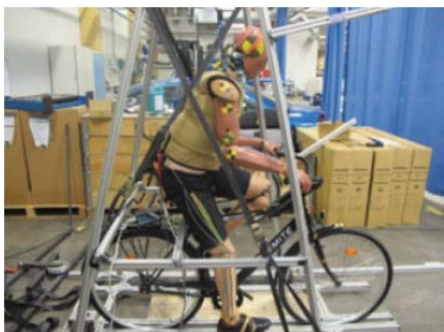
Figure 2: Cyclist impact testing using a Polar II crash test dummy (left). Three different impact scenarios (right) were evaluated in a study Fredriksson et al. (2014).
