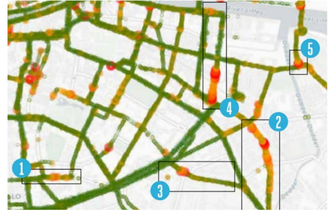
Data recorded by the See.Sense lights was used to get a better understanding of a Cities cycle network in terms of: Desire Lines, Junction Delay, Pavement Condition & Conflicts.
